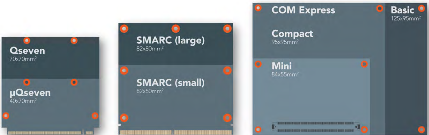
Comparing Qseven - SMARC & COM Express Source congatec (picture related to previous page)
